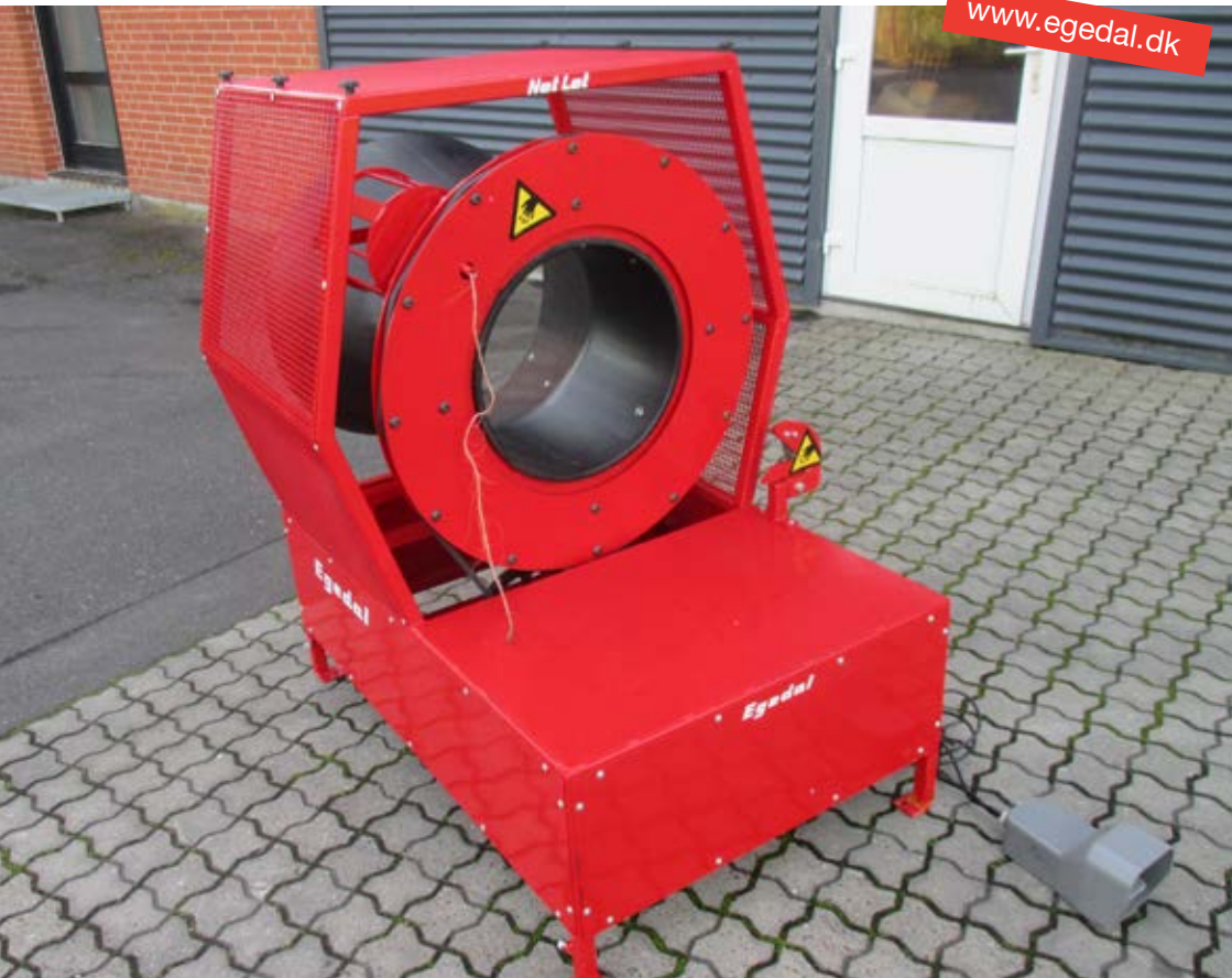
The tree is pulled through the funnel while the twine runs around the tree
