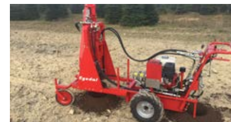
Bare-root plants and pots, hydraulically driven, drill sizes Ø10-Ø25 cm, drilling depth up to 300 mm, adjustable depth stop
