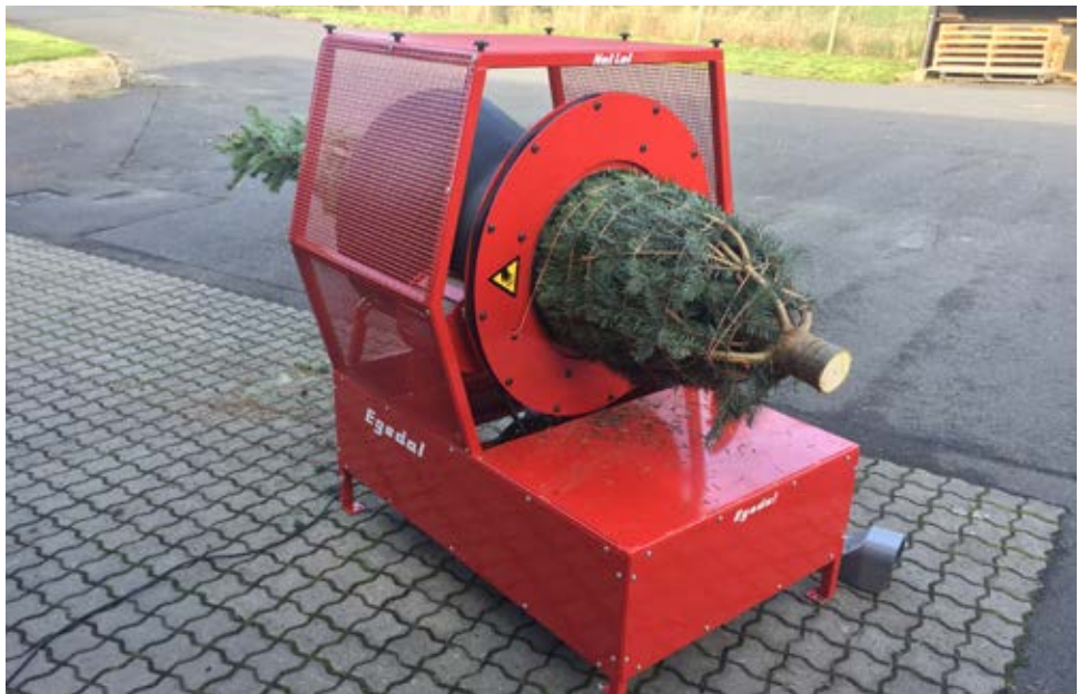
The tree is pulled through the funnel while the twine runs around the tree
